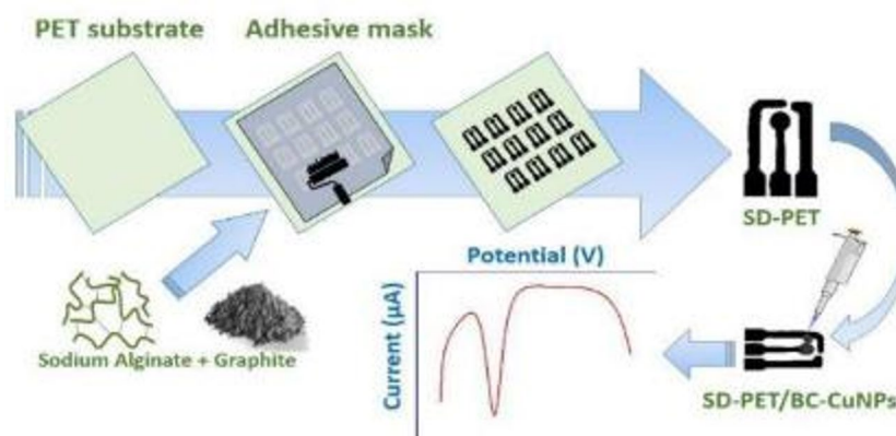
Fig. 1 Schematic flowchart illustrating the step-by-step fabrication of the disposable sensors: from the preparation of the PET substrate and adhesive masks, through the formulation of the graphite/sodium alginate conductive ink, to the manual screen-printing process, final surface modification with the BC-CuNPs composite via drop-casting, and the resulting DPV sensing profile for paraquat
