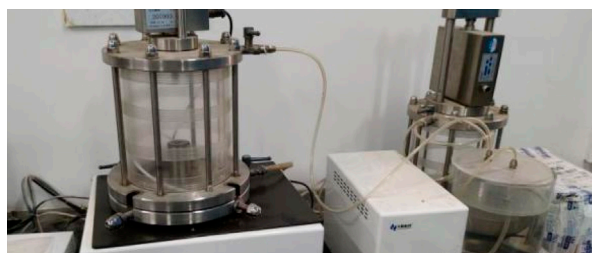
FIGURE 2 CU tri-axial loading system (MCU automatic hydraulic tri-axial apparatus).
