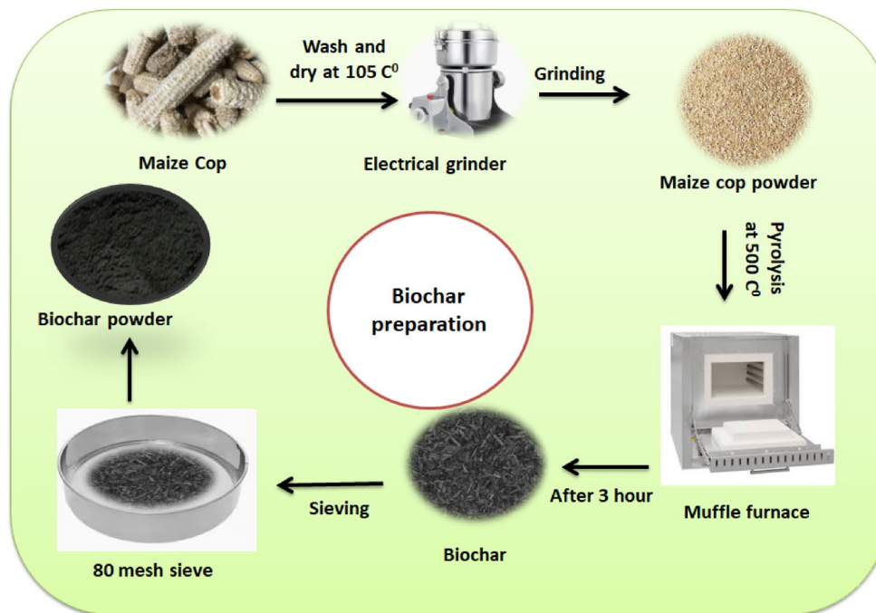
Scheme 1. Preparation of biochar with thermal method using muffle furnace at 500 °C.
