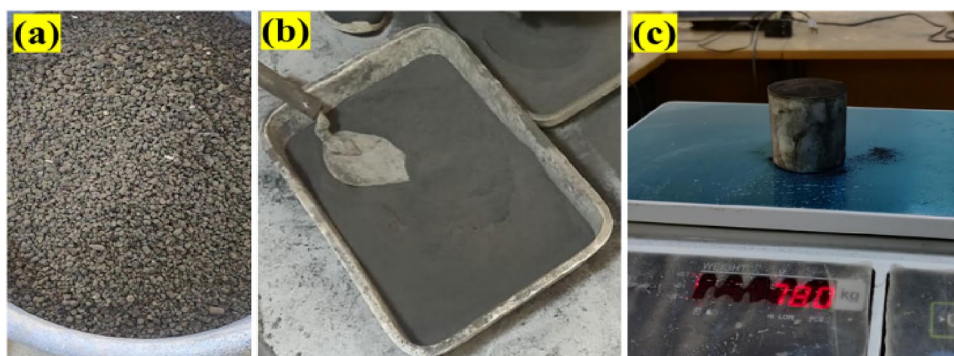
Fig. 3 (a) Raw biochar received from site; (b) processed biochar after grinding and sieving; (c) bulk density measurement of biochar.
