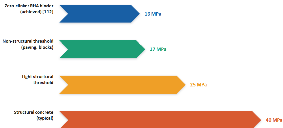
Fig. 8. Where a 16 MPa clinker-free binder fits
