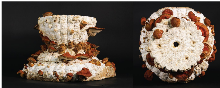
Fig. 13 Demonstrator after more than 28 days of air drying, fruiting bodies emerged: no visible contamination
