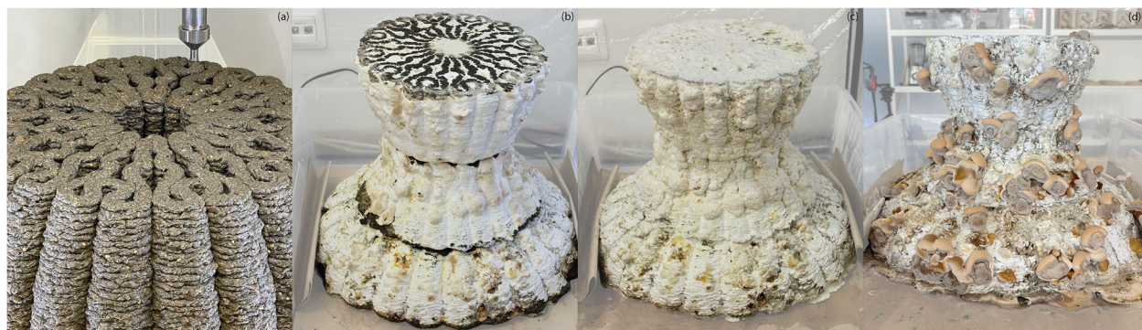
Fig. 11 Process timeline for the demonstrator: a freshly printed composite with reaction–diffusion toolpaths; b segments positioned after colonization over 14 days; c 7 days after, the elements are welded together biologically, ready for final drying, after which the piece behaves as a single element; d 28 days after, the connections are solid, being dried at room temperature to keep self-healing properties
