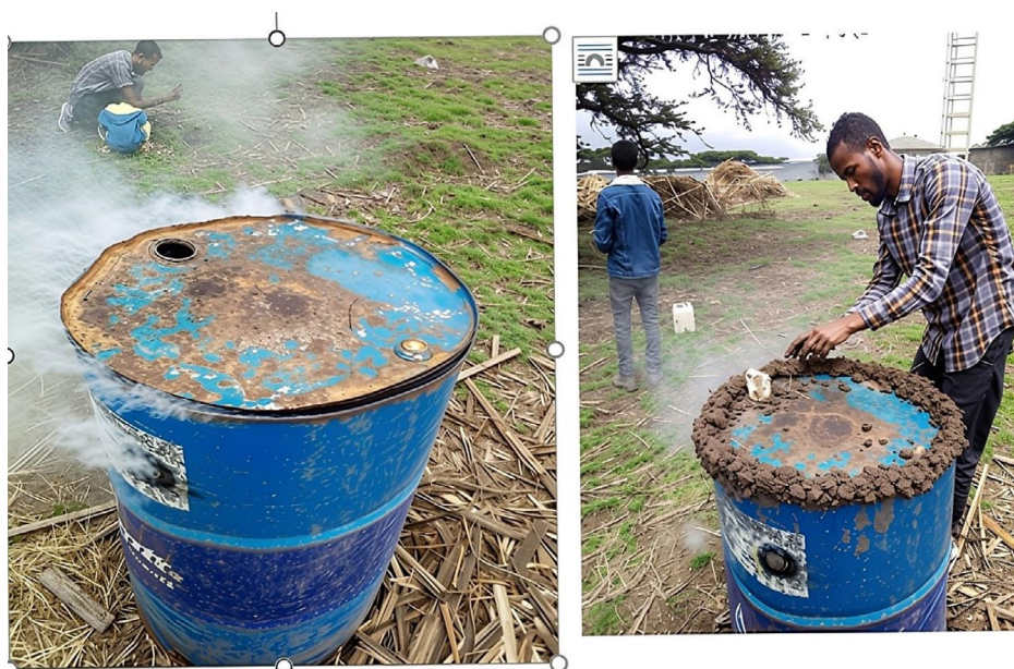
FIGURE 2 | This photo illustrates the biochar preparation process using metal vessels. On the left, a person monitors the setup, while on the right, another adjusts the metal barrel. The smoke indicates pyrolysis, where biomass is heated in low oxygen to create biochar, a sustainable method that enhances soil fertility and promotes carbon sequestration.
