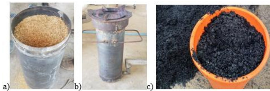
Fig. 2 Rice husk in the stove (a), Burning rice husk gasifier stove (b), Produced rice husk biochar (c)
