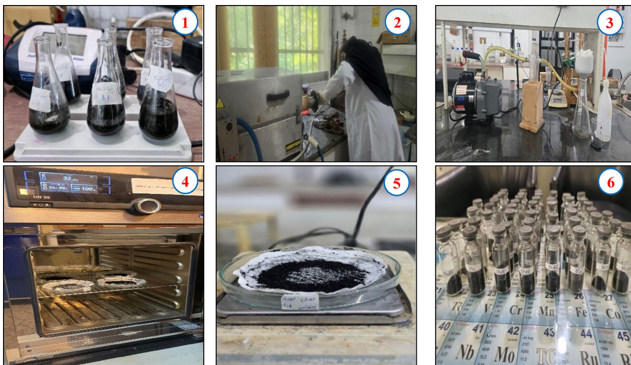
Fig. 3 Steps for preparing Morph-Genetic Porous Carbon (MGPC) from biochar, including 1) Diluting with distilled water, mixing and drying five grams of biochar with appropriate amounts of KOH or H_3PO_4 , 2) Injecting argon gas in a furnace at a temperature of about 800 °C for some 5 to 8 h, 3) Washing samples with distilled water and adjusting pH with nitric acid or sodium hydroxide solutions, 4) Drying the final samples in the oven, 5) Weighing the final samples, and 6) Sending prepared samples for BET analysis
