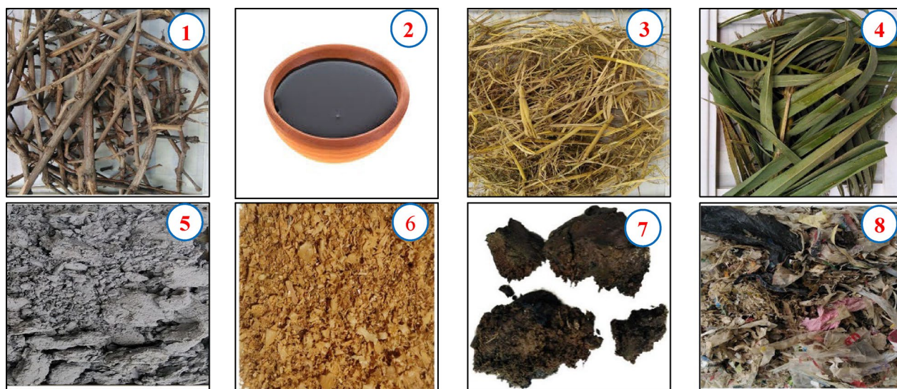
Fig. 2 Raw materials for biochar production, including 1) Vineyard pruning waste, 2) Vinasse, 3) Rice straw, 4) Vineyard pruning waste, 5) Tissue paper factory waste, 6) Sawdust, 7) Poultry slaughtering waste cake, and 8) Paper factory waste
