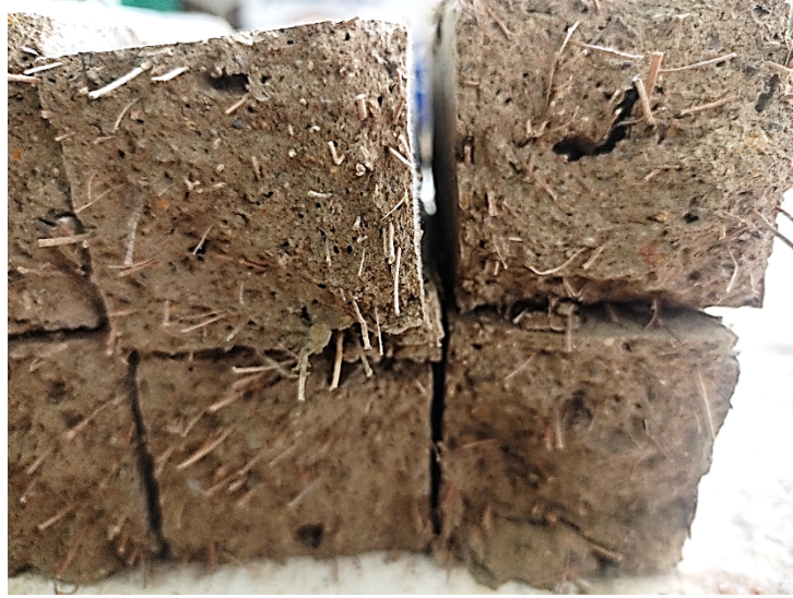
Fig. 7. Fracture surfaces of adobe bricks reinforced with biochar and Vicia faba fibres.
