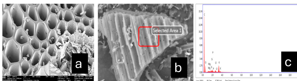
Figure 1. Scanning electron microscope micrographs a) micropore on cross section maize biochar, b) side view of maize biochar revealing micro channels and nano pore connecting micro channels, c) EDS for surface elemental analysis in selected area 1 depicted in 1b.
