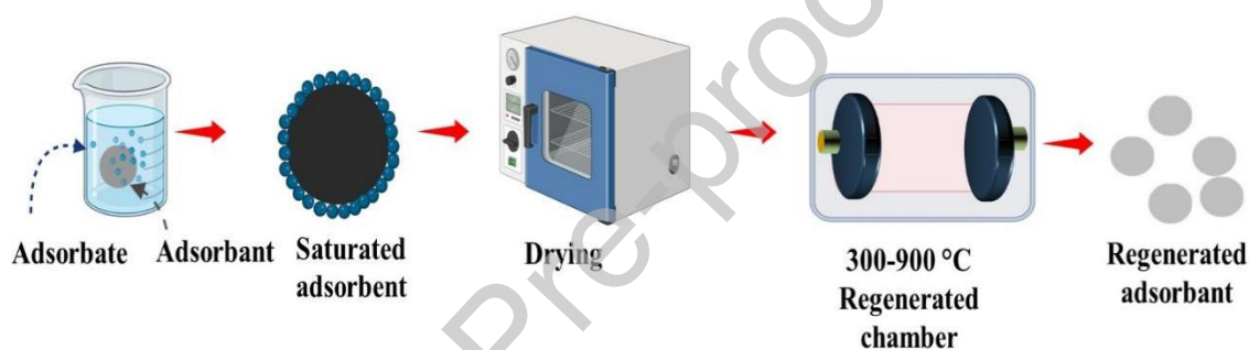
Fig. 16. Schematic of thermal regeneration.
