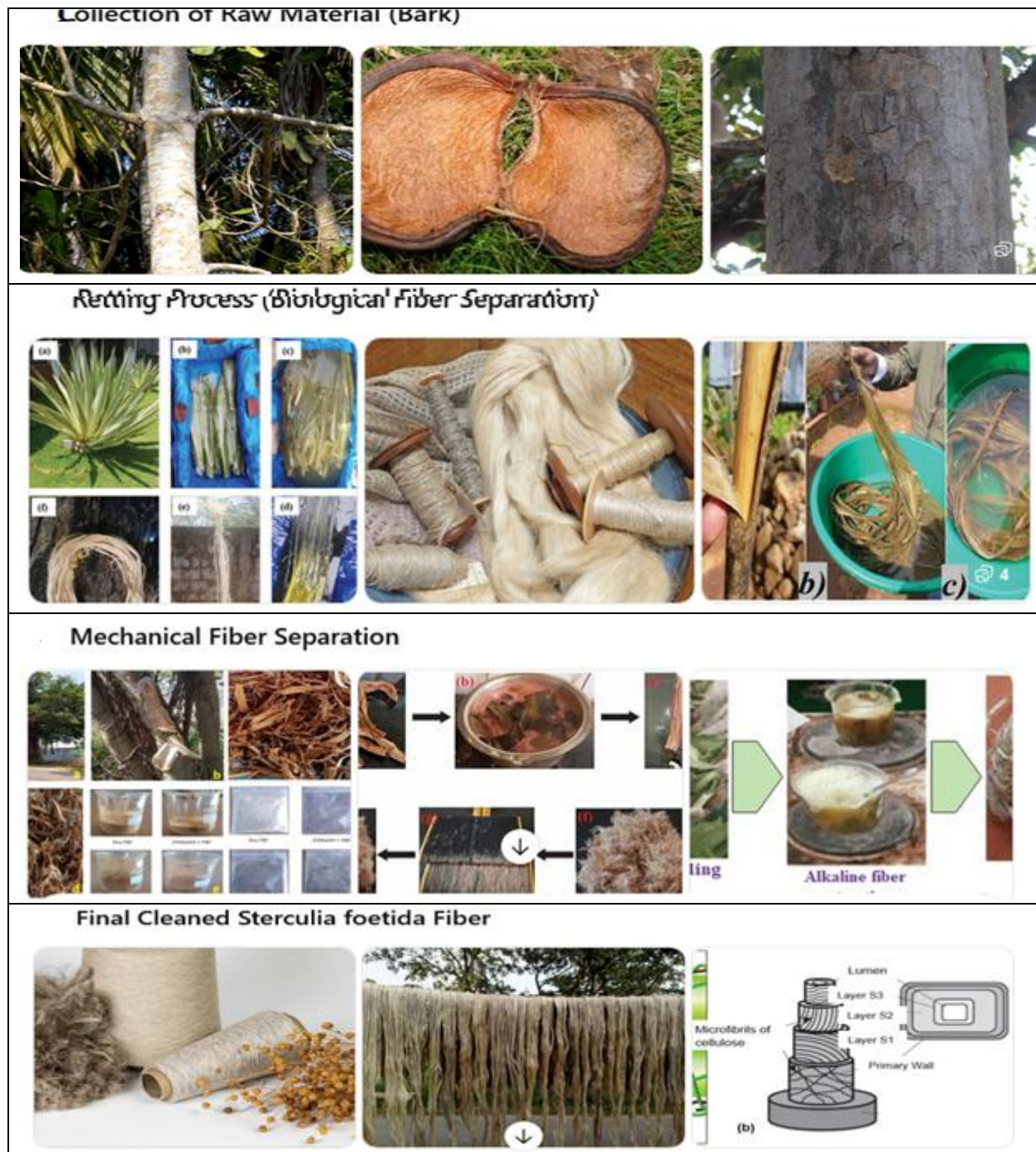
Fig-2: Sterculia- foetida Fiber Extraction Process
