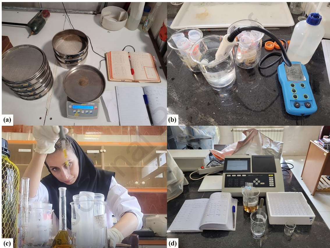
222 Figure 5. Investigation of soil changes before and after biochar application by measurement of aggregate mean 223 weight diameter (MWD) (a), soil pH and electrical conductivity (EC) (b), organic carbon (OC) content (c) and 224 chlorophyll-a content (d). 225 226
