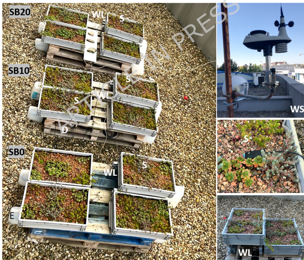
Fig. 1. Experimental setup installed on the rooftop of the Faculty of Education (Trnava University in Trnava, Slovak Republic). Plots contain roofing substrates without (SB0) and with the addition of 10% (SB10) and 20% (SB20) sewage sludge biochar (v/v). S - moisture/temperature sensor; D - datalogger; E - canister for runoff collection; WL - weighing lysimeter setup; WS - weather station.
