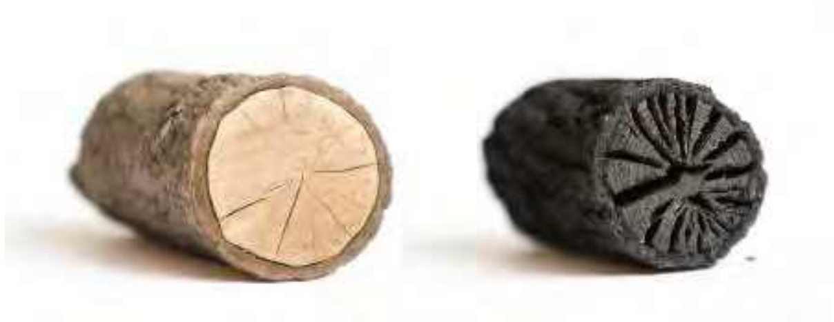
Figure 2 Example of woody feedstock from logging residues and resulting biochar. Photos: Daniel Albert
