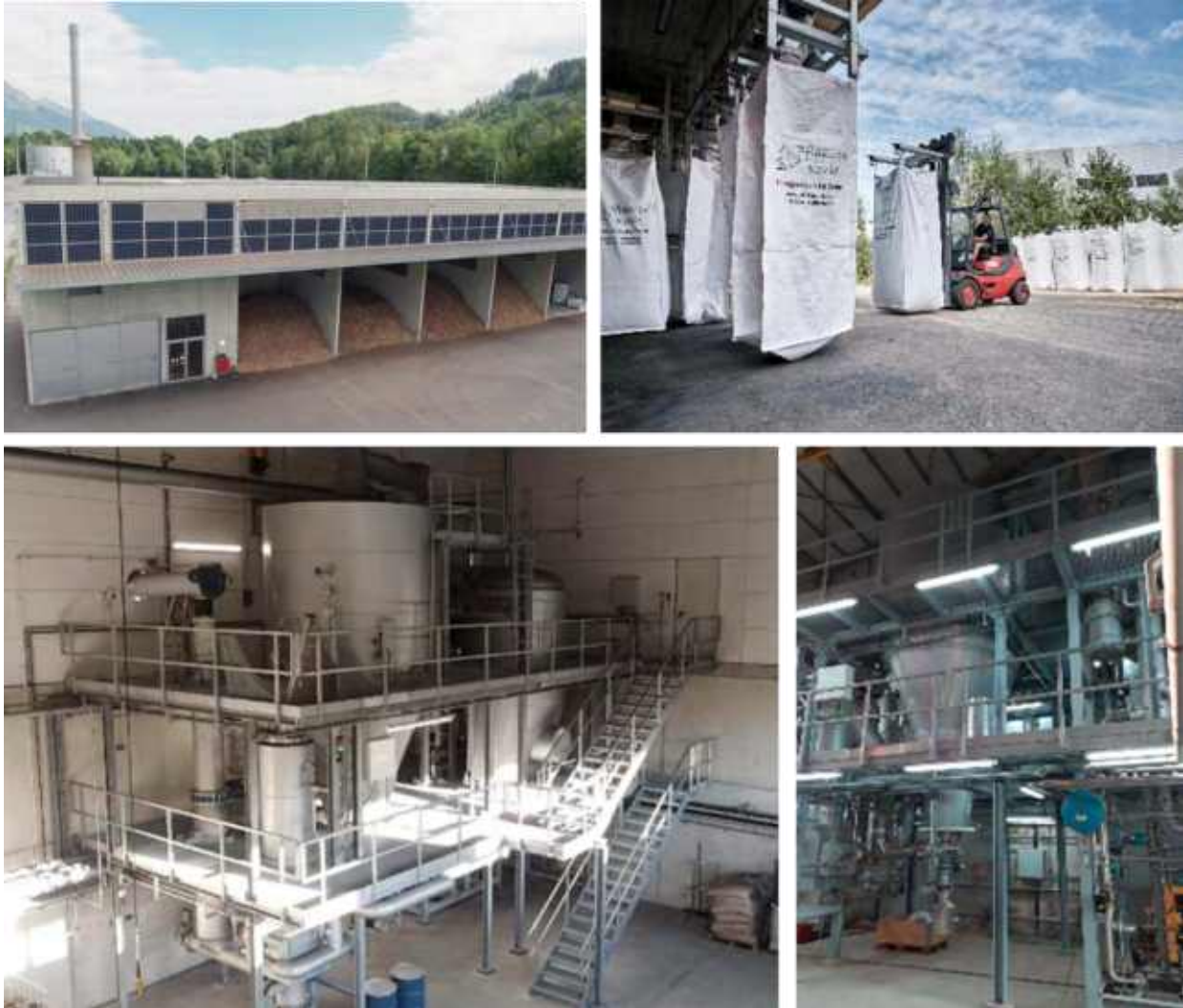
Figure 7 Examples from an industrialized biochar production facility. Feedstock storage (upper left), biochar filling into big bags (upper right), and reactor hall with conversion unit (below), Photos: Syncraft
