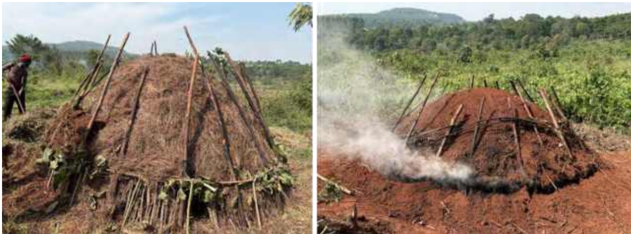
Figure 4 Traditional charcoal production in earth mound kilns in rural Uganda. Photos: Kathrin Weber
