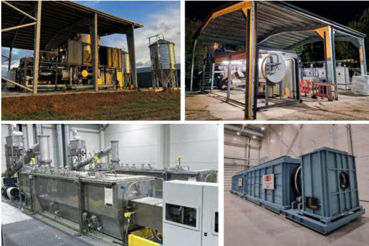
Figure 5 Examples of industrial biochar production. Upper left and right: Pyreg technology (Photos: Pyreg) Bottem left: Biogreen technology, bottom right: CHE technology (Photos: VOW)
