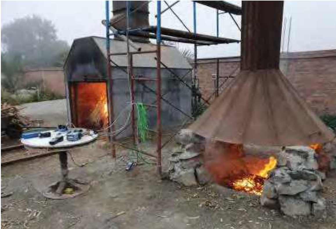
Figure 9 El Horno and flame curtain kilns, with the same principle. Emission measurements in Lima, Peru, published in [103]. Photos: Gerard Cornelissen
