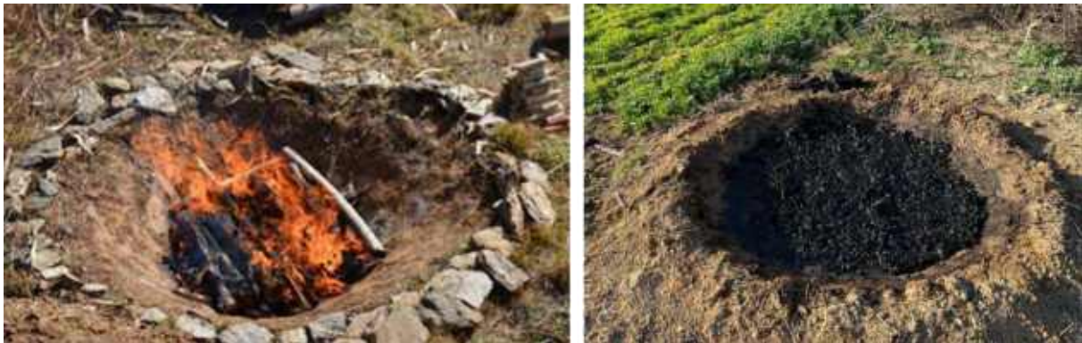
Figure 8 Conical Kon Tiki soil pit for cheap, clean, fast and easy artisanal biochar making. Photos: Gerard Cornelissen (left), Kathrin Weber (right)
