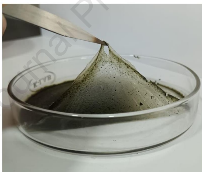
Fig.6. Synthesis of Bioplastic from Spirulina biomass residues
