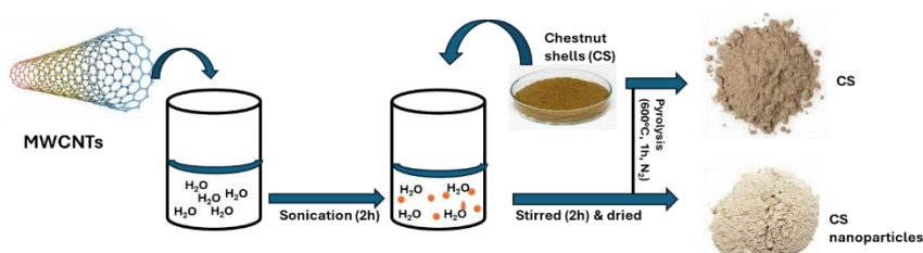
Figure 7: Schematic for the synthesis of biochar samples.
