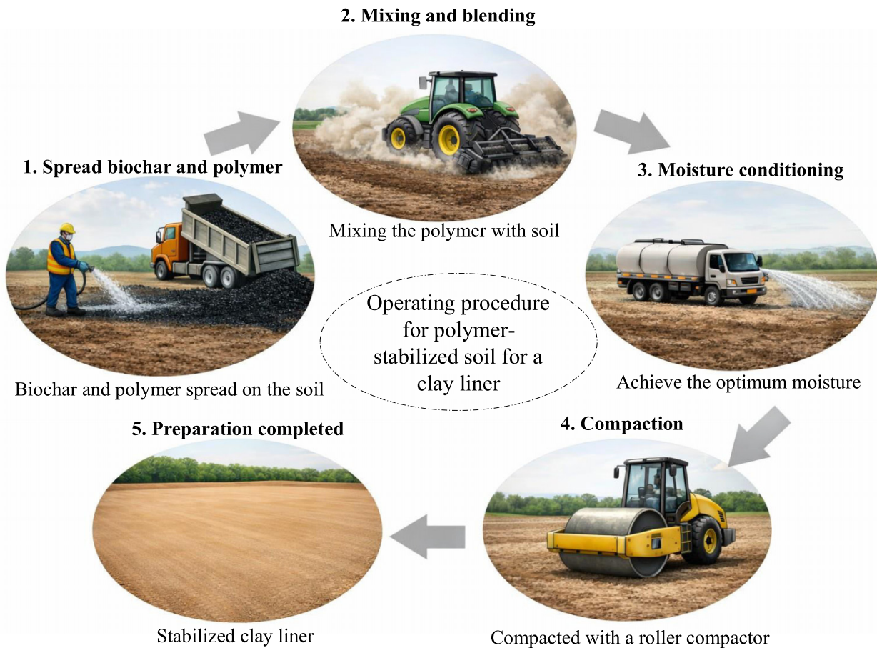
Fig. 15. Schematic illustration of a representative field-scale operating procedure for the application of bis(2-hydroxyethyl) terephthalate polymer for soil stabilization.
