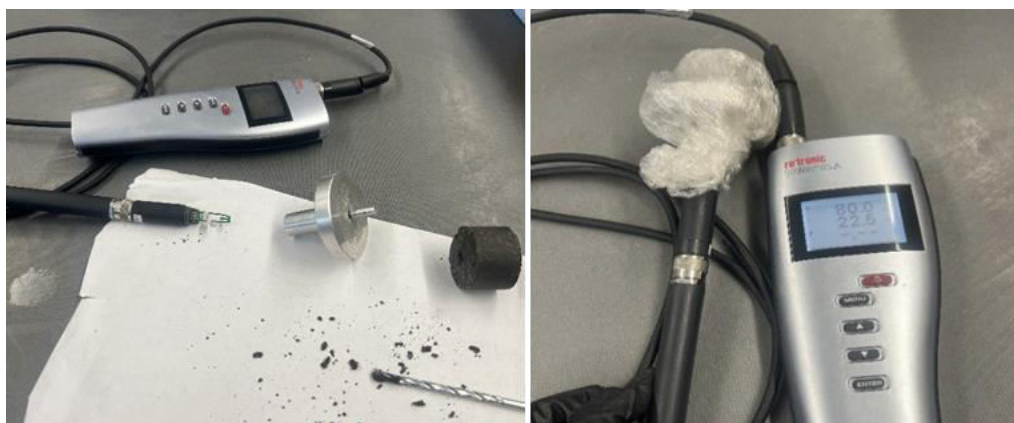
Fig. 3. Suction tip and relative humidity sensor to measure relative humidity.
