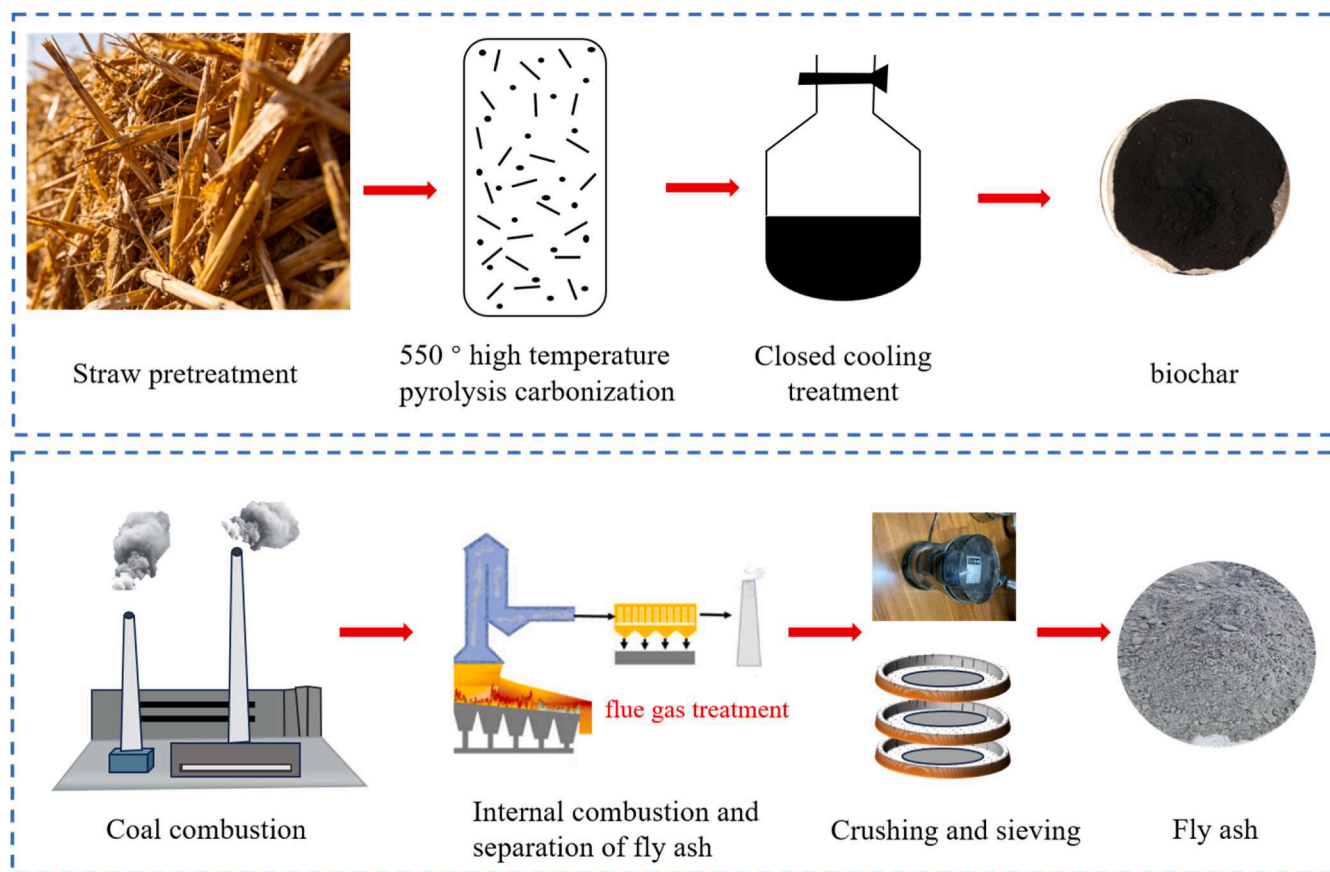
Fig. 2. Process flow of biochar preparation and the harmless recovery of fly ash.
