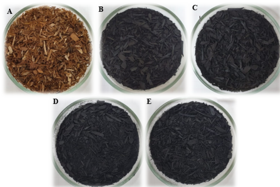
Figure 3. (A) CE—raw Eucalyptus bark; (B) B300; (C) B350; (D) B400; (E) B450—biochar samples produced at increasing pyrolysis temperatures.
