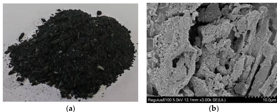
Figure 1. Physical appearance and microstructure of the corn straw-derived biochar. (a) Macroscopic view of the biochar particles used in the study; (b) scanning electron microscope (SEM) image revealing the porous surface structure.
