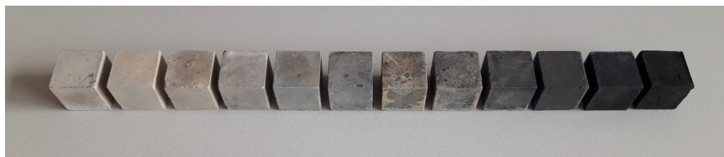
Figure 5. Alkali-activated slag composites with carbon-based BW made from wood waste, prepared in order to determine compressive strength (sample numbers increase from left to right).
