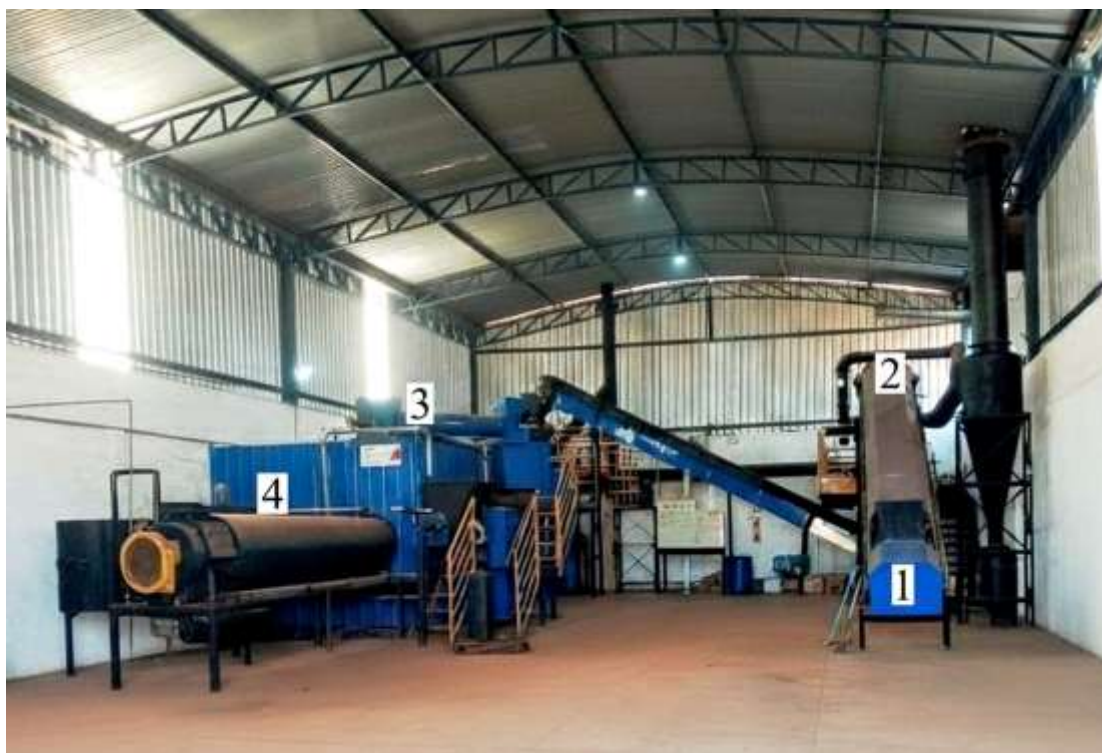
Figure 1. The system operates with continuous feed via a conveyor belt, integrating (1) a manual biomass feeding unit, (2) a drying section, (3) a pyrolysis reactor, and (4) cooling of the solid product.
