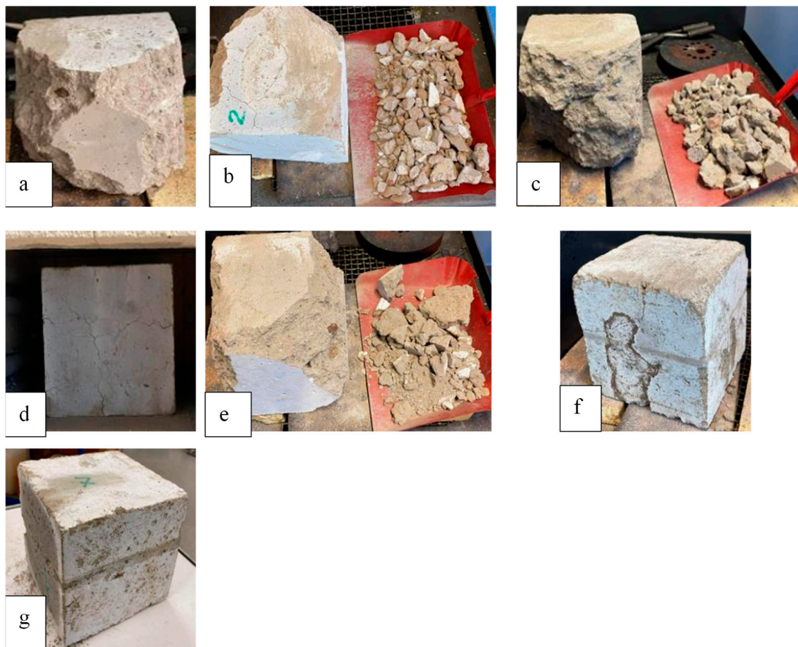
Figure 14. (a–g) Visual documentation of post-fire cracking for all recipes (R1–R7).
