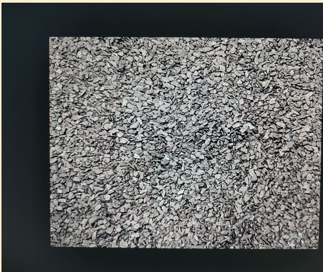
Photo 1. Raw biochar from cocoa pod shell biomass (Pyrolysis temperature: 400°C ; degradation time: 1 hour). Photo Y. G. L. Koffi.
