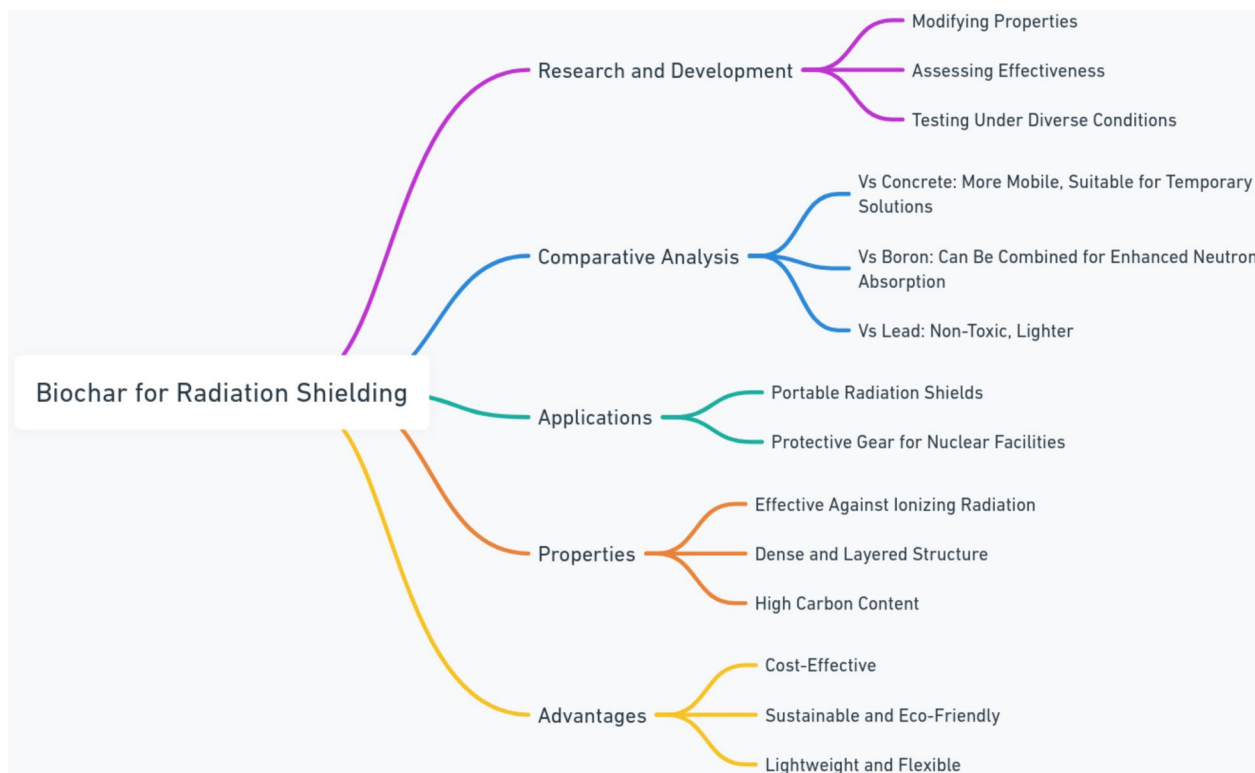
Fig. 5 Innovative radiation shielding with biochar: properties, R&D process, and comparative analysis (Martellucci and Torsello 2022; Barbhuiya et al. 2024)
