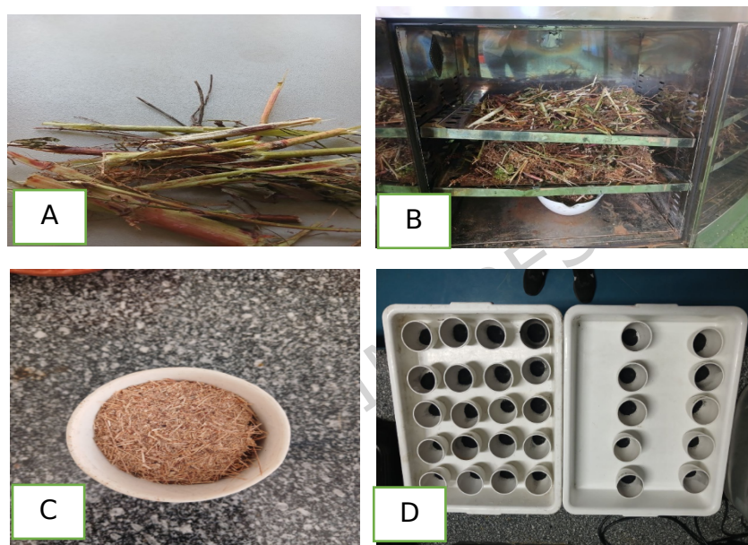
108 Figure 1. Preparation Stages of Biochar: (A) Steam treatment of Rumex abyssinicus , (B) 109 Oven drying, (C) Grinding, and (D) Synthesized biochar experimental runs
