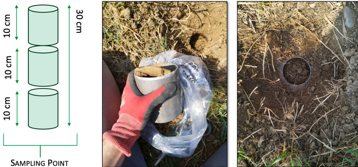
Fig. 3. Metal ring method used in sampling 30 cm topsoil.
