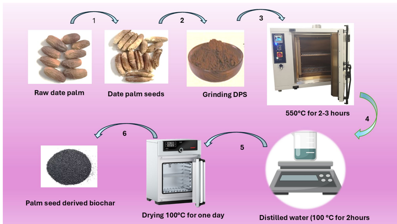
Fig. 1 The steps of synthesized phoenix dactylifera seed-derived biochar
