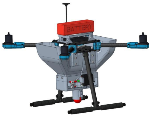
(a) Conceptual design with seed mechanism in gray.
