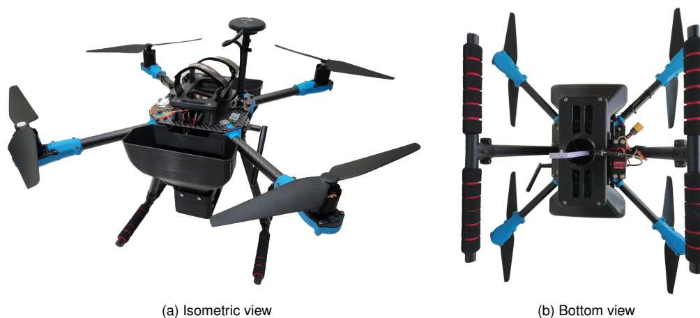
Figure 5: Final prototype with full integration of seed-dropping mechanism on HolyBro X500 V2 platform.
