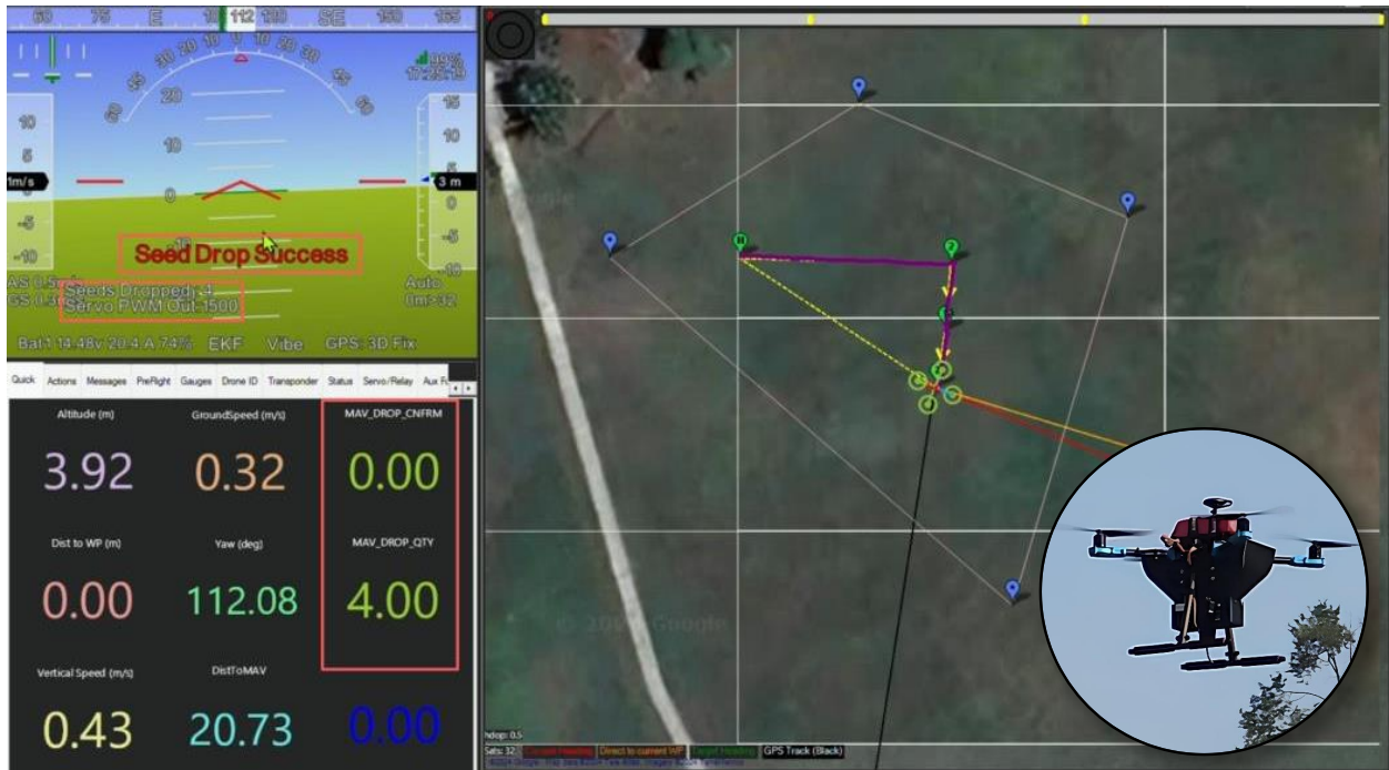
Figure 12: Autonomous mission trajectory and initial field test of the UAV seed-dropping system. Waypoints are marked in green, geofence is outlined with blue markers, and UAV trajectory is shown in purple. Lua script provides feedback of seed drops to operator via the dashboard (highlighted with orange boxes).
