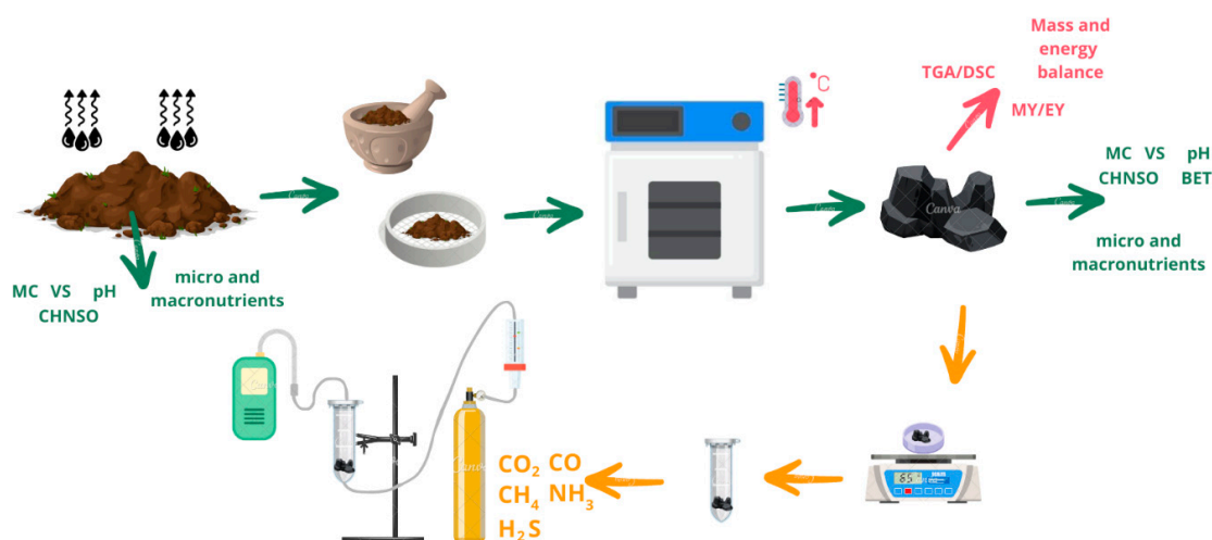
Figure 4. (a) Compost samples and compost biochar. (b) Experiment setup: configuration for the process of producing biochar from compost (green line), schematic diagram of adsorption test (yellow line), and mass and energy balance (red line).
