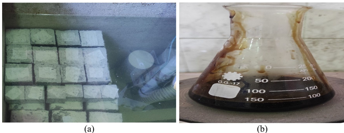
Fig. 3. (a) Mixing and curing water, and (b) the used SP (Sikament NN).
