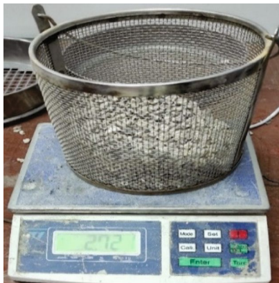
Fig. 2. (a) Particle size distribution of sand, (b) particle size distribution of dolomite, (c) crushing test of dolomite, and (d) absorption test of dolomite.
