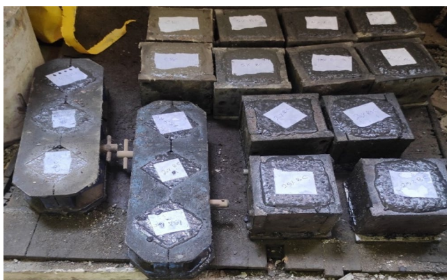
Fig. 5. Sample of RHB mortar and concrete cube specimens.
