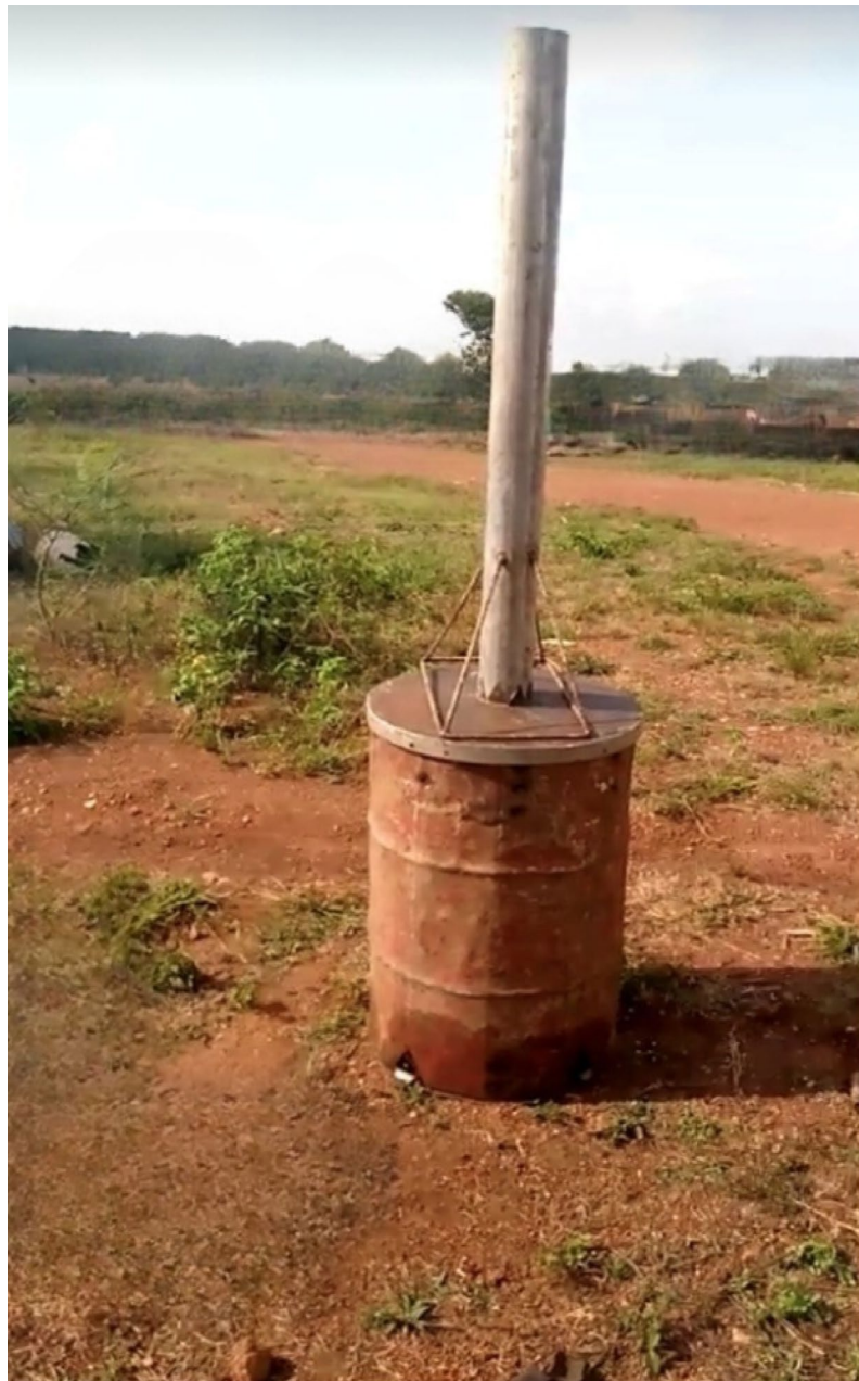
Fig. 1. A locally fabricated metal drum kiln used for biochar production through pyrolysis.
