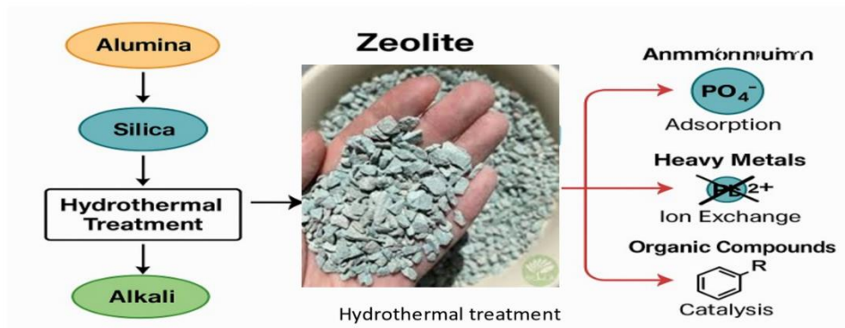
Figure 4. Zeolite synthesis and application
