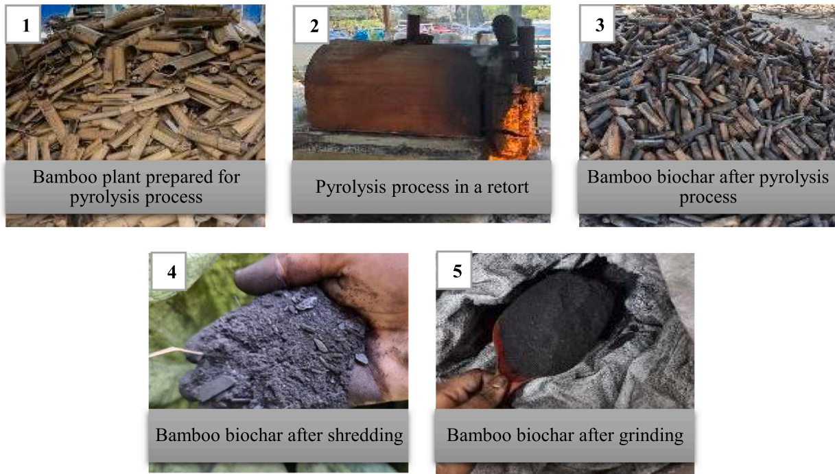
Fig. 1. Bamboo biochar process flow using pyrolysis method.
