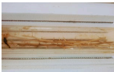
Fig. 2. Pyrolysis process of P. Juliflora sample: The biomass is subjected to thermal decomposition in a tube furnace under controlled conditions to produce biochar.
