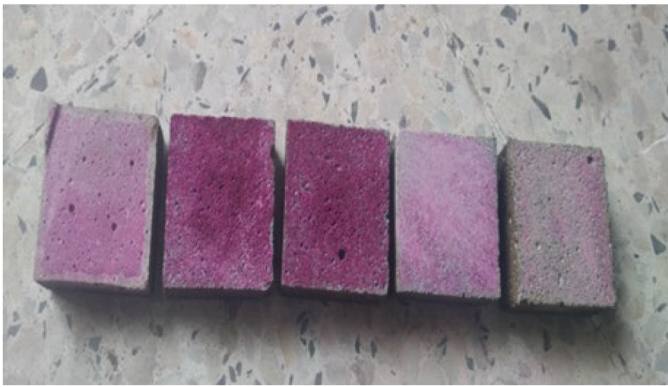
Fig. 17. This image shows five concrete specimens after the phenolphthalein carbonation test, arranged from right to left in order of increasing biochar content (0, 0.05, 0.1, 0.15, and 0.2 wt%). Pink regions indicate uncarbonated areas (high pH), while colorless areas represent carbonated zones (low pH due to \text{CO}_2 reaction).
