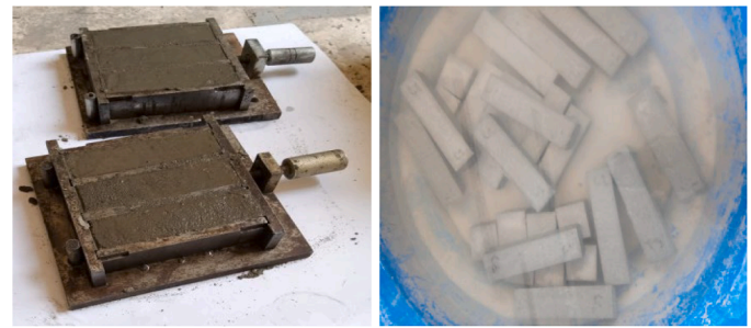
Fig. 4. Processes involved: (Left) Sample casting process showing the filling of molds with mortar and preparation for initial setting. (Right) Sample curing process in a water bath maintained at 25 \pm 1^\circ\text{C} to ensure proper hydration and strength development.
