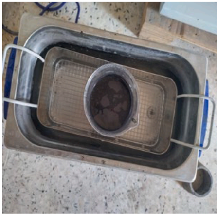
Fig. 5. Sonication process of biochar: Ultrasonic waves are applied for 30 min to disperse biochar uniformly in 80 % of the calculated water, ensuring effective integration into the mortar mix.
