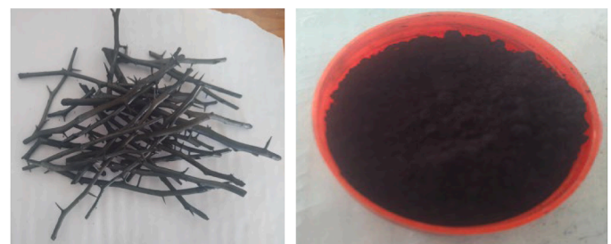
Fig. 3. Biochar preparation: (Left) Pyrolyzed biomass showing the raw material after thermal decomposition. (Right) Fine biochar obtained after grinding and sieving, ready for incorporation into the mortar mix.
