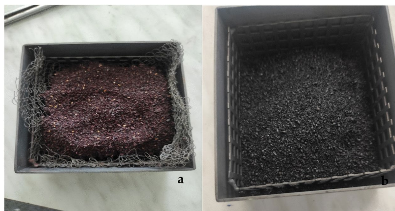
Fig. 1. (a) chokeberry before pyrolysis process, (b) biochar from chokeberry after pyrolysis process in 500 °C.
