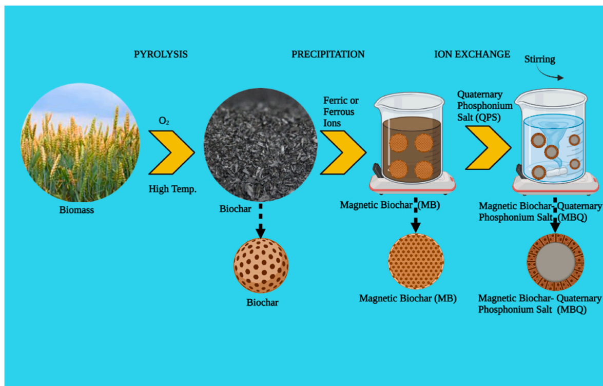
Fig. 4. Complete process of preparation of magnetic biochar-quaternary phosphonium salt [MBQ].
