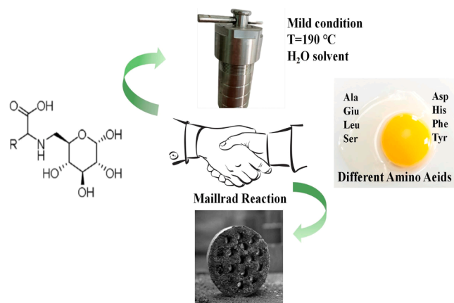
Fig. 6. Schematic mechanism of N-rich hydrochar synthesis from egg white biomass in the presence of sucrose (see Vahdati-Khajeh 2019, Surfaces and Interfaces).
