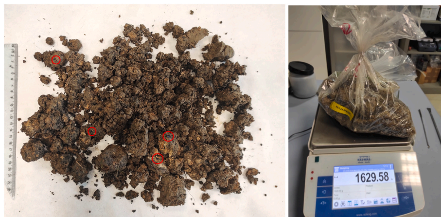
Fig. 6. Biochar-containing soil sample (left - visible biochar particles in red circles) and weight of one soil sample (right). (For interpretation of the references to colour in this figure legend, the reader is referred to the Web version of this article.)
