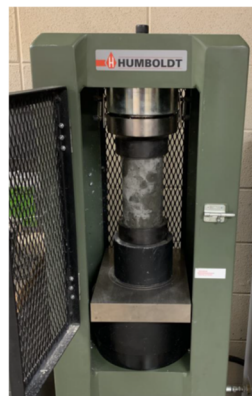
Figure 6. Compressive Strength Testing of Biochar Metakaolin Concrete.
