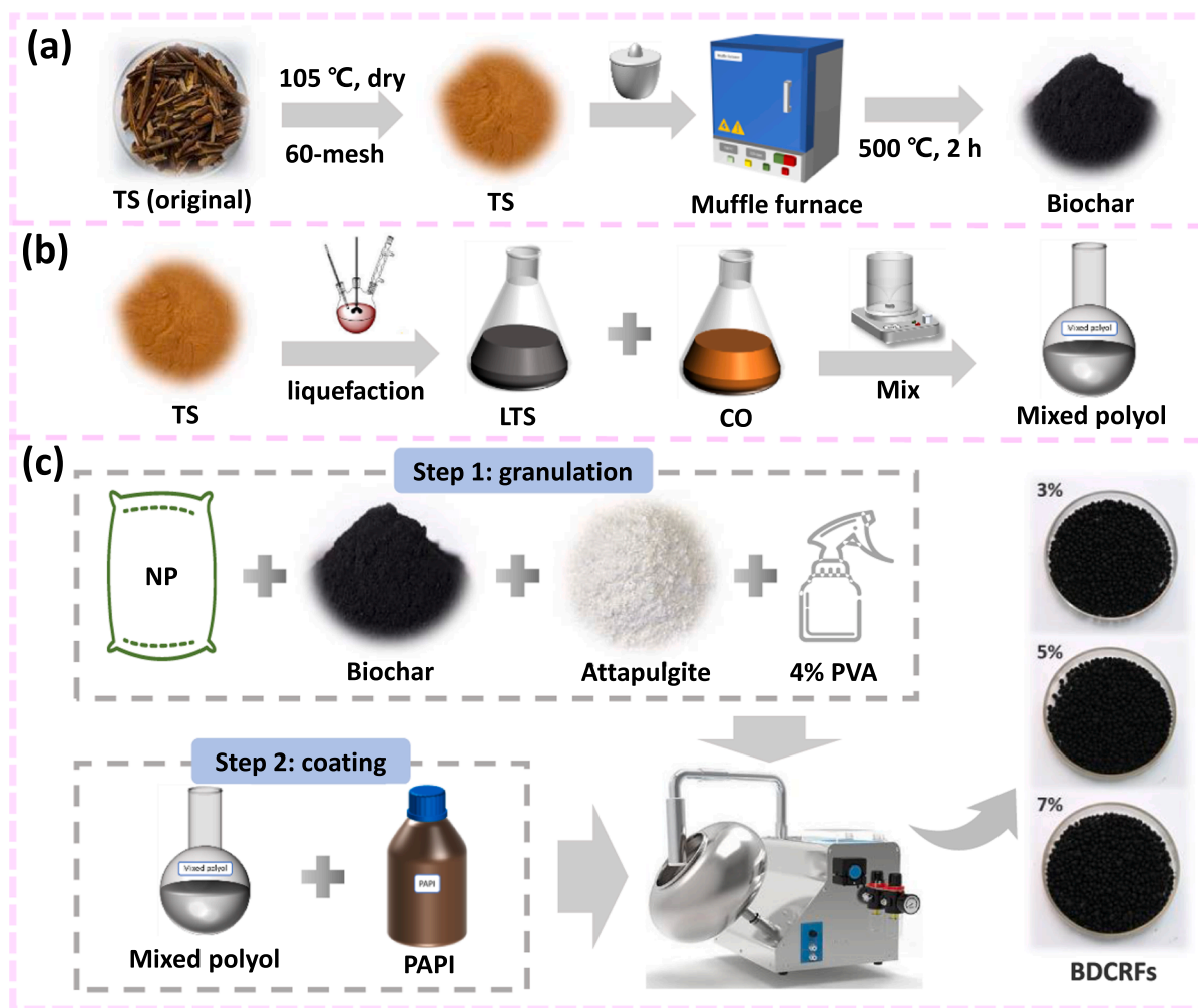
Fig. 1. The scheme of preparation progresses for (a) biochar, (b) mixed polyol, (c) BDCRFs.
