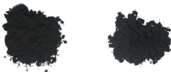
(a) Sludge-based biochar; (b) Waste wood-based biochar
