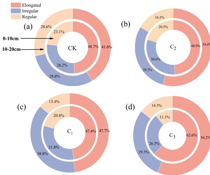
Fig. 6. Effect of biochar on soil pore shape distribution. Note: CK (Control), C 1 (7.5 t ha -1 ), C 2 (15 t ha -1 ), and C 3 (30 t ha -1 ). (a) soil pore shape distribution of CK; (b) soil pore shape distribution of C 1 (c) soil pore shape distribution of C 2 (d) soil pore shape distribution of C 3 .
