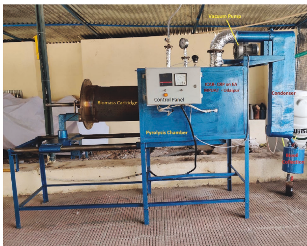
Figure 2. The pictorial view of Vacuum Pyrolyzer Instruments.
