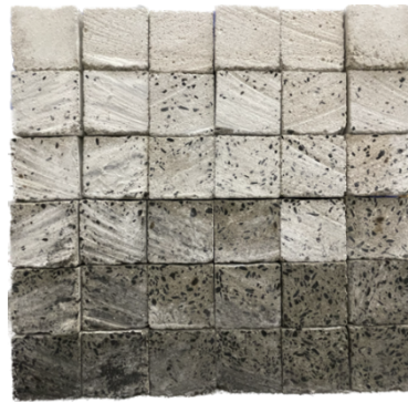
Fig. 20: Cross section of the PCM-biochar loaded cement at different sand replacement.
