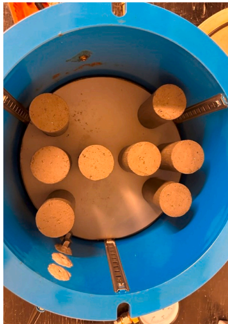
Fig. B2. Stabilized samples placed in the carbonation chamber.
