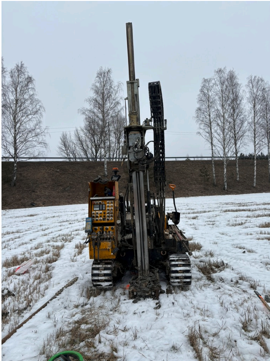
Fig. A2. The machinery used to obtain the clay samples from different depths.
